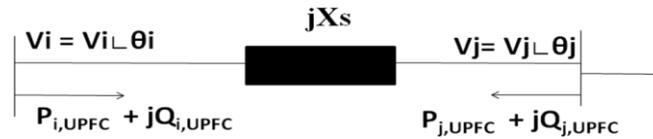
Fig :3 Power injection model of UPFC
